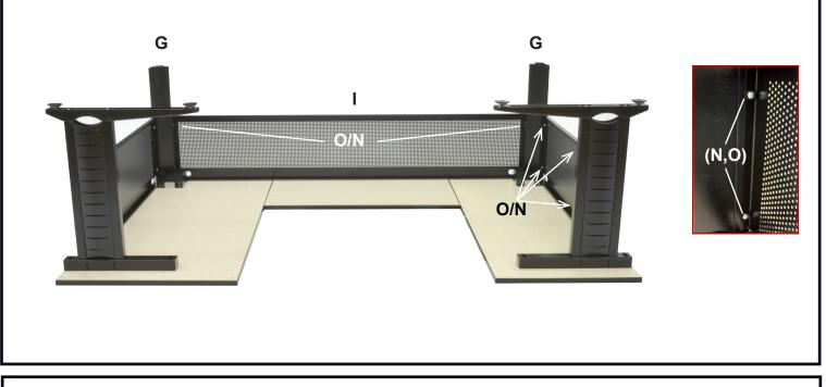
**STEP 8:** Square the legs and modesties using a tape measure. Arrange all metal components so there is an equal margin on the top/bottom & left/right sides. Connect the **End Legs** and **Corner Legs(G)** to the tops as *figure 1* and 2 depict. For extra support connect the Short Modesties(J) to the table top using 2 Screws(Q) each modesty.
